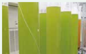
Algae culture (photosynthesis) using sunlight and CO 2 released from a cement factory
