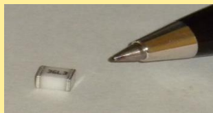
Smallest-class surge absorber for power supply
