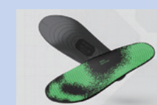
Insole-type sensor (industrial accident prevention insole)
