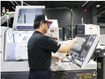
Mr. Enami checking a machining tool capable of supporting the LFV technology
