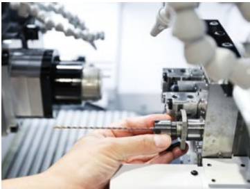
DVAS attached to a machine tool allows for the drilling of tiny, deep holes.
