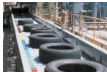
Waste tires, plastics and oil used as a fuel substitute in cement plants
